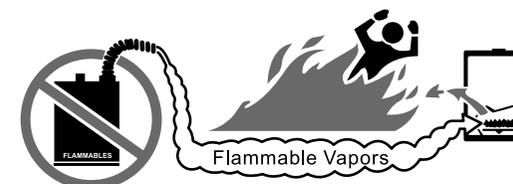
**Vapors from flammable liquids will explode and catch fire causing death or severe burns.** Do not use or store flammable products such as gasoline, solvents or adhesives in the same room or area near the water heater.
