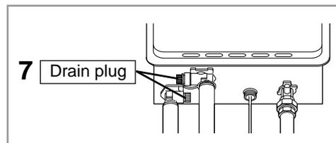
8 When the water is completely drained, replace all drain plugs and close the hot water fixtures.
