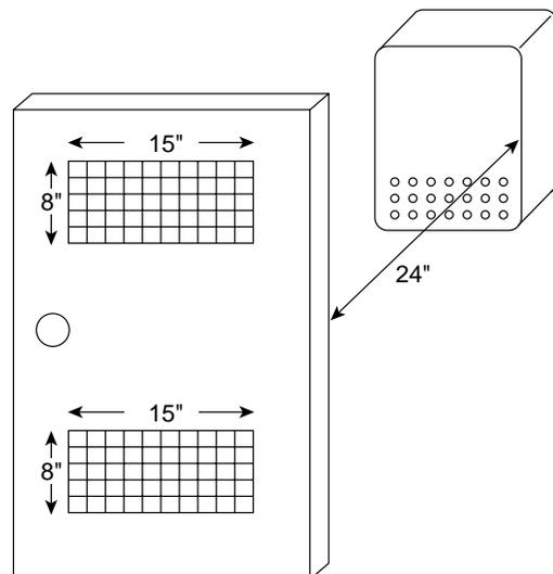
To install the water heater in a kitchen or a room with a duct, a volume of air intake equivalent to the volume of air going out through the duct is needed, so as not to reduce the air pressure in the room.
